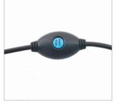
The blue pairing button can also be used to lower the base to the flat position in case of an emergency (see battery backup section on pages 23 – 24).
